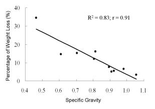
Fig. 4 Correlation of specific gravities and percentages of weight loss of coconut blocks tested
