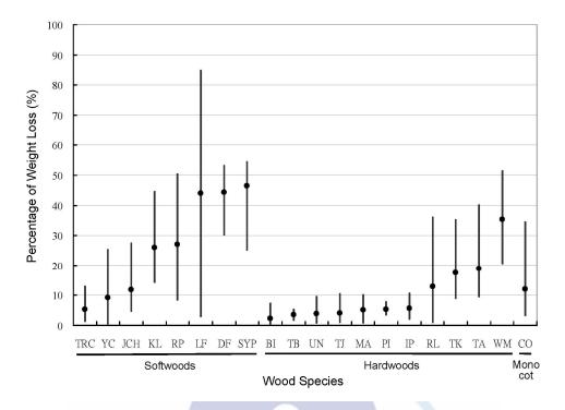
Fig. 1 Averages and ranges of percentage of weight loss of replicate blocks of the 20 wood species tested
