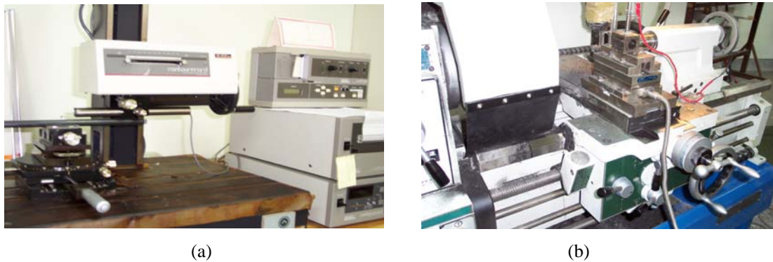
Fig.4 The experimental set-up (a) surface roughness measuring, (b) dynamometer, tool and GFRP workpiece.
