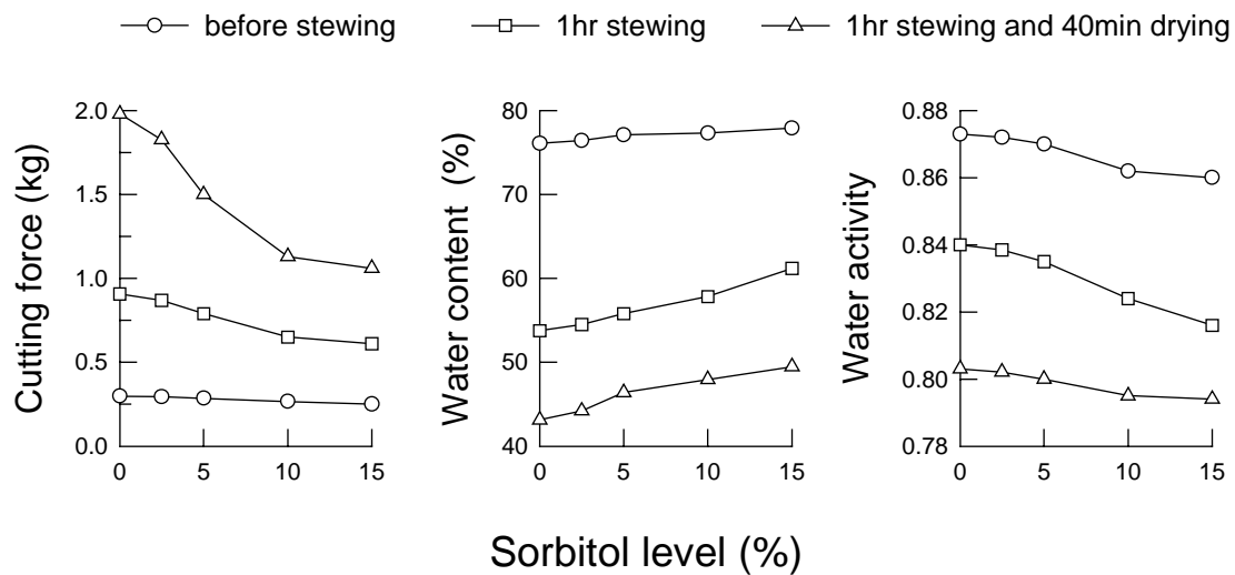
1 圖三 添加0.5%血漿蛋白及不同量的山梨糖醇的魚香腸佃煮1小時後在70 熱風 2 乾燥過程中剪切力、水分含量及水活性的變化 3 Fig.3. Cutting force, water content and water activity of fish sausage sections made 4 from horse mackerel surimi with 0.5% plasma protein and different level of 5 sorbitol
