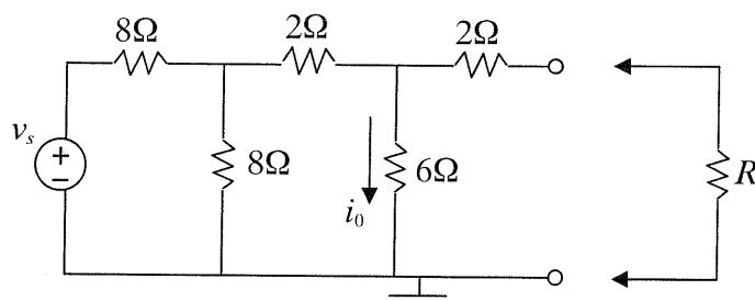
3. (20%) Find the Norton equivalent circuits with respect to terminals  $a$  and  $b$ .
