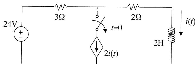
5. (20%) Consider the following third-order circuit with input voltage  $v(t)$ . Write the state equation  $\dot{x}(t) = Ax(t) + b v(t)$ , where  $x(t) = [x_1(t) \ x_2(t) \ x_3(t)]^T$  contains three state variables  $x_1(t)$ ,  $x_2(t)$  and  $x_3(t)$  shown in the circuit.
