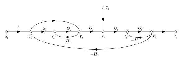
Fig. 2. Signal Flow Graph
