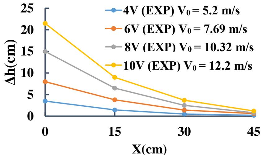
Fig. 7 Comparisons of experimental  $\Delta h$  estimated from the variation of inlet flow velocity.
