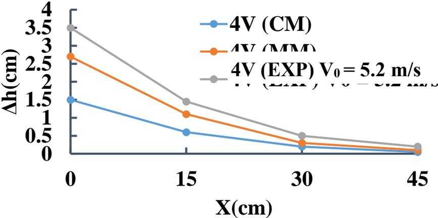
Fig. 5 Comparisons of  $\Delta h$  estimated from classical model (CM), modified model (MM) and experiment (EXP) while the inlet flow of 5.2 m/s is specified.
