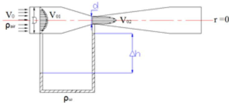
Fig. 2 The diagram of venturi manometer
