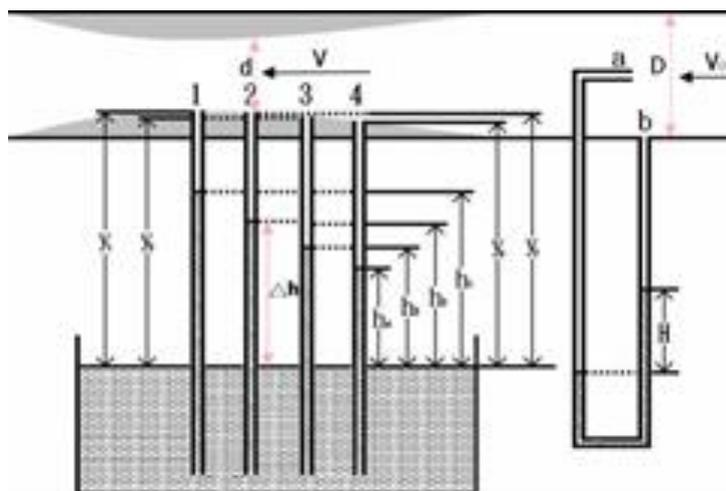
Fig. 4 The outlines of dynamical and static pressure gauge.
