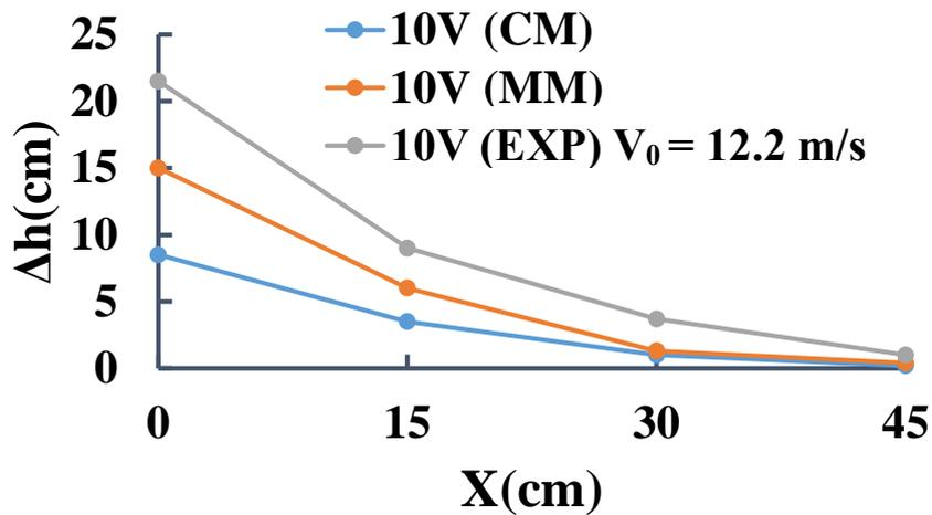
Fig. 6 Comparisons of  $\Delta h$  estimated from classical model (CM), modified model (MM) and experiment (EXP) while the inlet flow of 12.2 m/s is specified.
