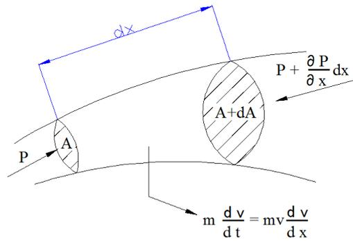
Fig. 1 Schematic of flow element
