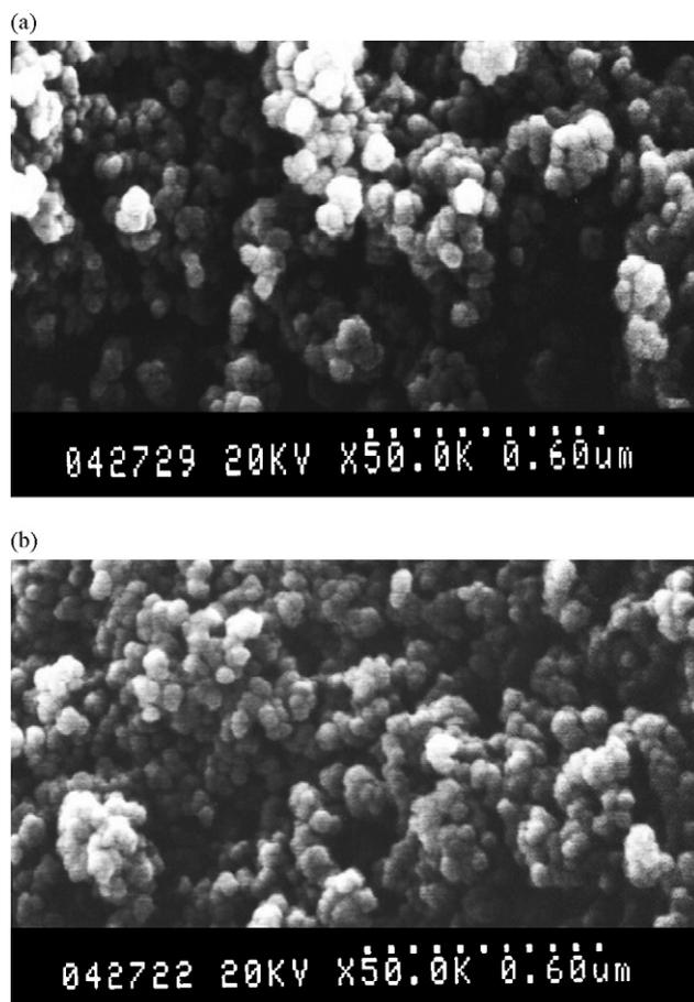
Fig. 3. Scanning electron micrographs of (a) TiO<sub>2</sub> and (b) Ag/TiO<sub>2</sub> (50,000 $\times$ ).
